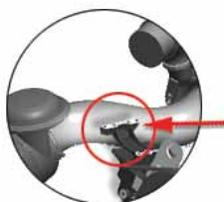
**Avoid mounting in areas where ducting is exposed to components that could cause abrasive wear.**
