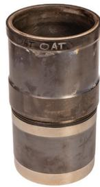
Thrust Side of Liner After Field Test
