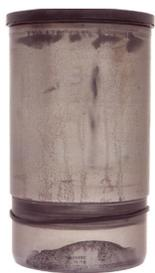
Thrust Side of Liner After JD Cavitation test
