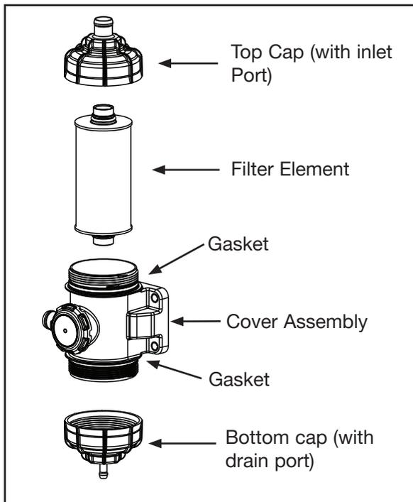
**Figure 5:** Exploded view of the CV filter housing
