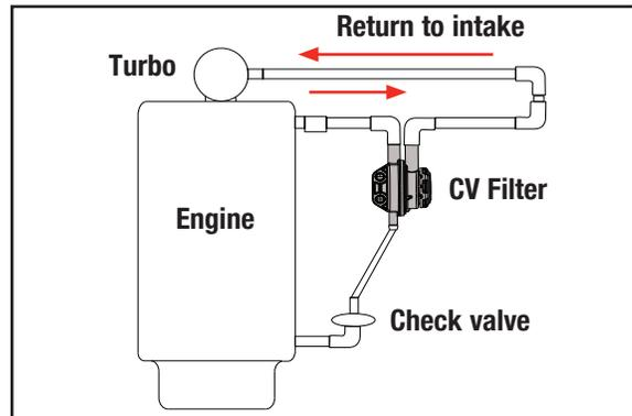
**Figure 4 - Diagram of a CCV system assembly - Arrows show flow direction.**
