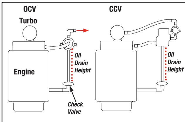
Figure 5- Setting the Oil Drain Height
