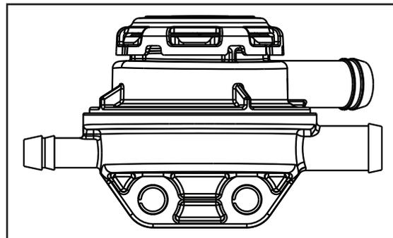
**Figure 2: Side view of CV Unit, showing mounting holes**
