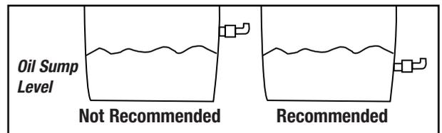
Figure 6: Oil drain port preferred location on the oil sump.
