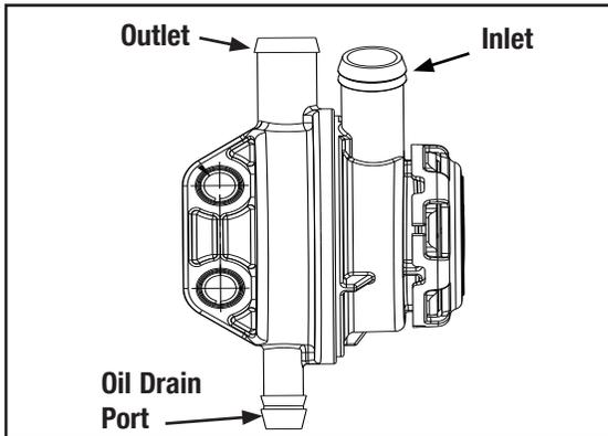
**Figure 1 - CV Unit Preferred Orientation: Oil Drain Port Pointing Down**
