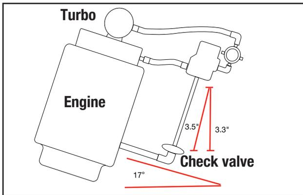
**Figure 7 - Effect of engine inclination on oil drain height**
