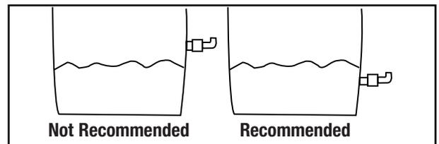
Figure 6: Oil drain port preferred location on the oil sump.
