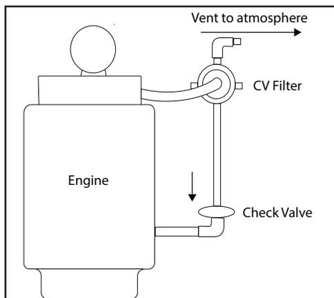
Figure 3: Diagram of a OCV system assembly - Arrows show flow direction.
