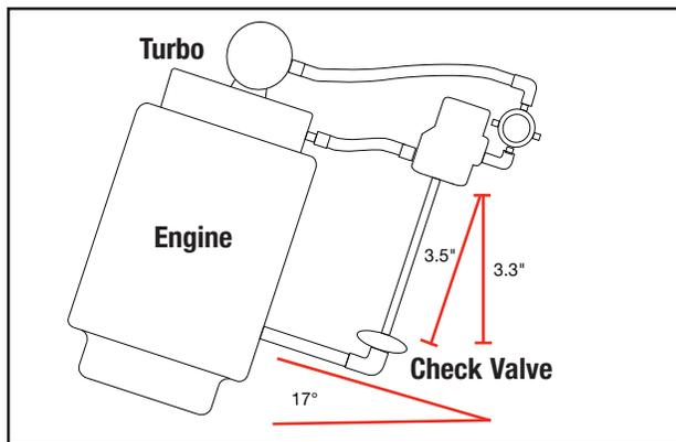
**Figure 7 - Effect of engine inclination on oil drain height**
