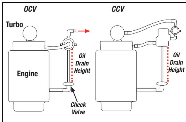
Figure 5 - Setting the Oil Drain Height
