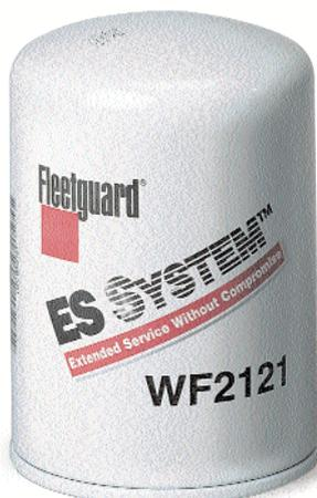
These ‘intelligent’ water filters contain Cummins Filtration patented slow release chemicals and are suitable for cooling systems up to 80 litre capacity. For larger cooling systems it is recommended to use (if fitted) a non-chemical coolant filter plus ES Extender liquid to maintain optimal cooling system protection.
