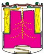
Non-soluble permeable coatings provide graduated (= slow) chemical release. Furthermore, clumping of the pellets slows down the full release.
