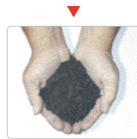
1g of dust ingested per engine horsepower is enough to destroy the engine
