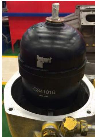
**Figure 7: CS41018 installed in Eliminator**
