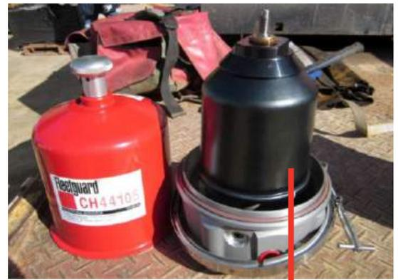
Figure 1: Remote Centrifuge housing
