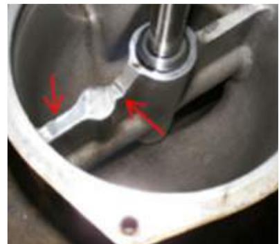
**Figure 8: Ensure Rotor Clears Gussets**
