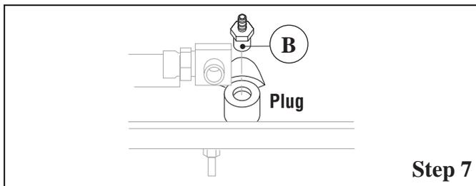
**Step 7** - Screw in the drain fitting and tighten until snug. **Do not overtighten.**
