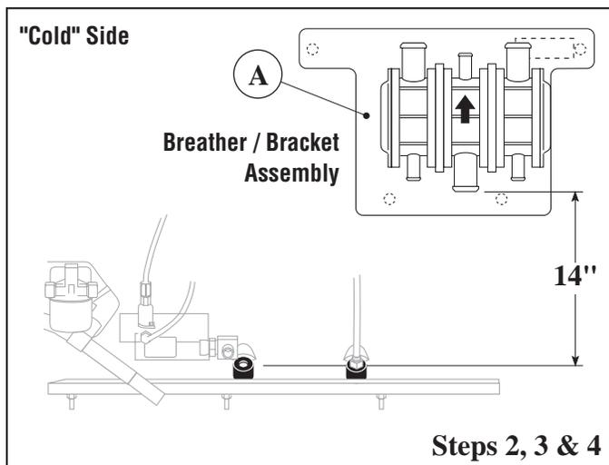
**Step 2** - Find a mounting location for the breather assembly and bracket at least 14 inches (350 mm) above the dipstick ports. The assembly must be a minimum of 4 inches (100 mm) from both the exhaust manifold and exhaust system components.
