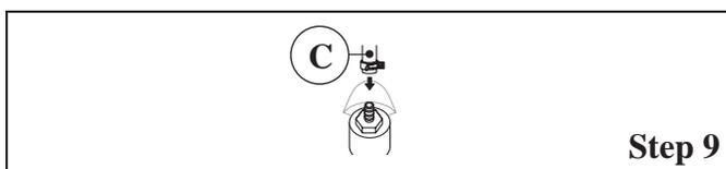
**Step 9** - Route the drain hose to the drain fitting assembly. **If the hose is too long, trim the excess from the end of the drain hose. Ensure the check valve in the drain tube assembly is in a vertical position. Do NOT cut off the check valve or any of the hose above the check valve. Secure with clamp. Reinspect the hose and routing to verify it is free of any loops, kinks or abrupt bends.**
