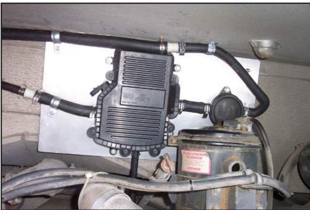
Figure 6 – Connecting the Coalescer Unit to the CDR Valve
