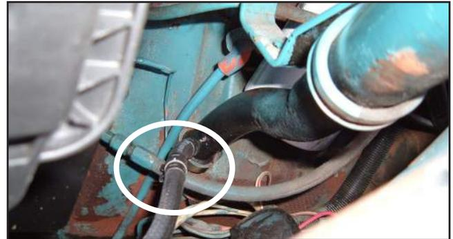
Figure 10 – A Barbed Hose Fitting Welded to the Bottom of the Oil Fill Tube for the Drain Back Location for the Drain Line
