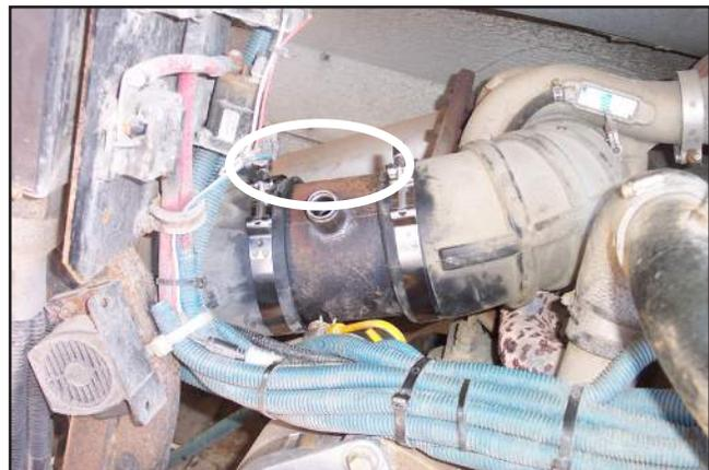
Figure 7 – 1" (25 mm) Hose Barb Welded to the Intake Piping for the Return Line
