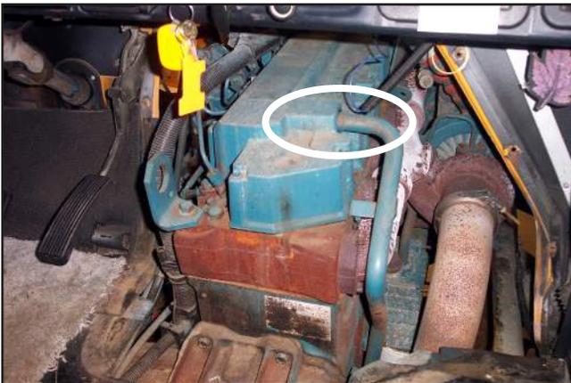
Figure 5 – Coalescer Inlet Connecting to Crankcase
