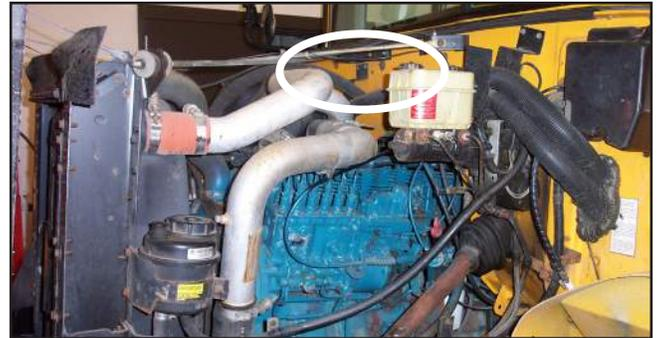
*Figure 3 – Possible Mounting Location for New Brackets in the Engine Bay*
